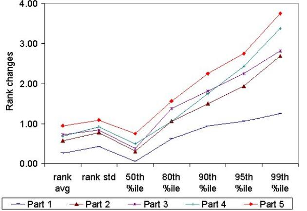
Figure 4: Rank changes of the top five most probable failed parts in Net 3 based on 100 run cases across different scenarios with CPT noise  $\epsilon \sim N(0, 1.0)$ .
