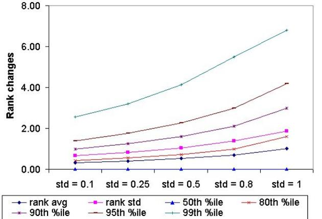
Figure 5: Rank changes of the most probable failed part in Net 1 based on 100 runs cases across different scenarios and prior noise.
