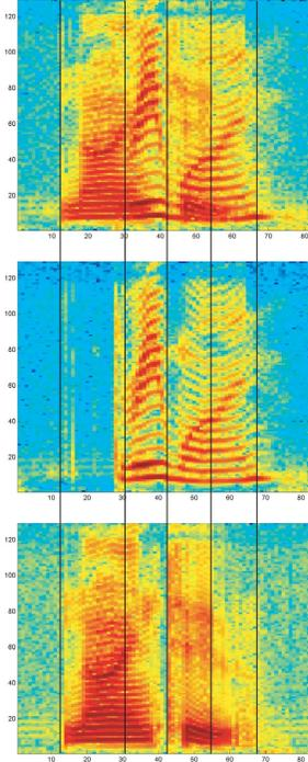
Figure 11: First pane shows the composed spectrogram, second and third spectrograms correspond to the individual sources, vertical lines correspond to the frames learned as states. Notice how the model captures the switches of dominant speaker.
