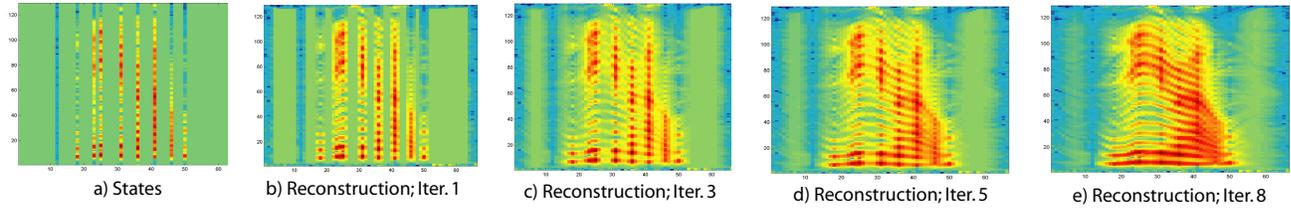
Figure 9: Reconstruction from the matching-tracking representation, starting with just the explicitly-modeled states, then progressively filling in the transformed intermediate states.
