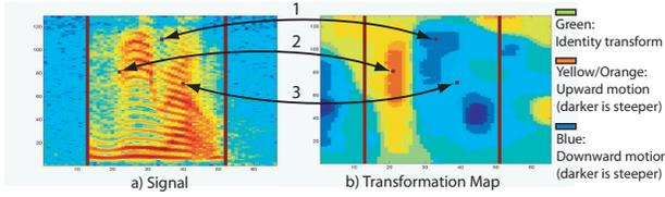
Figure 4: Example transformation map showing corresponding points on original signal.
