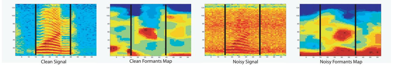
Figure 7: Formant tracking map for clean speech (left panels) and speech in noise (right panels).
