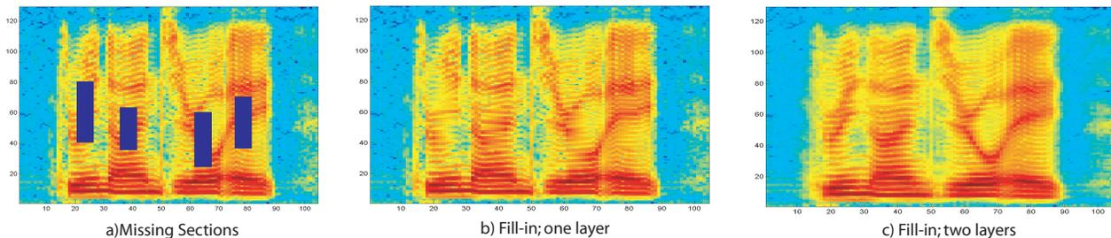
Figure 6: (a) Spectrogram with deleted (missing) regions. (b) Filling in using a single-layer transformation model. (c) Results from the two-layer model.
