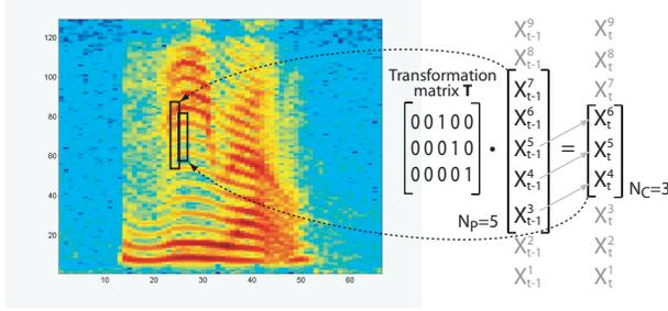
Figure 1: The  $N_C = 3$  patch of time-frequency bins outlined in the spectrogram can be seen as an “upward” version of the marked  $N_P = 5$  patch in the previous frame. This relationship can be described using the matrix shown.
