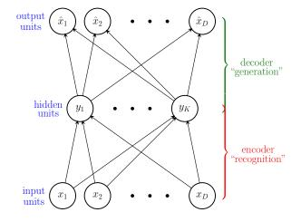
Given a set of N observed "input" vectors  $\{\mathbf{x}_n\}$ , the weight matrices P and Q are set to minimise the "autoencoding error"  $\sum_n \|\hat{\mathbf{x}}_n - \mathbf{x}_n\|^2$ , often using iterative gradient descent. Assume the input vector distribution has zero mean.
