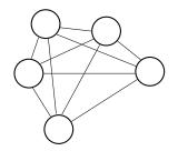
Undirected graphical model (i.e. a Markov network) over a vector of binary variables  $s_i \in \{0,1\}$ . Some variables may be hidden, some may be visible (observed).
