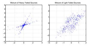
These distributions are generated by linearly combining (or mixing) two non-Gaussian sources.
