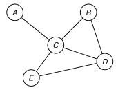
An **undirected graphical model** is a direct representation of conditional independence structure. Nodes are connected iff they are conditionally dependent given all others.
