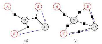
Conditional independence:  $X \perp\!\!\!\perp Y \mid \mathcal{V}$  if **every** path between X and Y contains some  $V \in \mathcal{V}$ .
