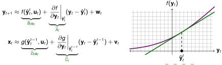
Run the Kalman filter (smoother) on non-stationary linearised system  $(A_t, B_t, C_t, D_t)$ :
