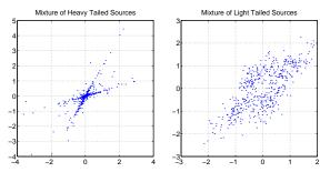
These distributions are generated by linearly combining (or mixing) two *non-Gaussian* sources.
