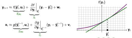
Run the Kalman filter (smoother) on non-stationary linearised system  $(\widetilde{A}_t, \widetilde{B}_t, \widetilde{C}_t, \widetilde{D}_t)$ :
