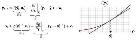
Run the Kalman filter (smoother) on non-stationary linearised system  $(\widetilde{A}_t, \widetilde{B}_t, \widetilde{C}_t, \widetilde{D}_t)$ :
