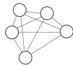
Undirected graphical model (i.e. a Markov network) over a vector of binary variables  $s_i \in \{0,1\}$ . Some variables may be hidden, some may be visible (observed).
