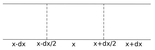
This is a bare-bones schematic; in addition to what's shown, there is an external current,  $I_e(x,t)$ , and a current associated with channels,  $I_m(x,t)$ .
