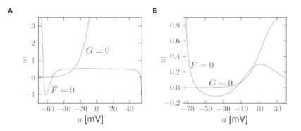
Figure 2: Copied from ND textbook fig. 4.3. A shows the nullclines of the Hodgkin-Huxley model rigorously reduced by setting  $m(t) = m_{\infty}(V(t))$  and fitting a linear function  $w(t) = c_h - h(t) = c_n n(t)$  such that  $c_h - h(t) \approx c_n n(t)$ . B shows the nullclines of the simplified Morris-Lecar model. As above, u = V on abscissa.
