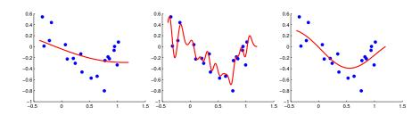
Kernel methods can control **smoothness** and **avoid overfitting/underfitting**.
