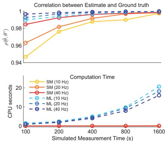
**Fig. 1.** Comparison between score matching (SM) and maximum likelihood (ML) estimation for the generalised linear Poisson model. SM achieves high correlation to ground truth (note the y-axis on the upper figure) and approaches the performance of ML with considerably lower computational cost.
