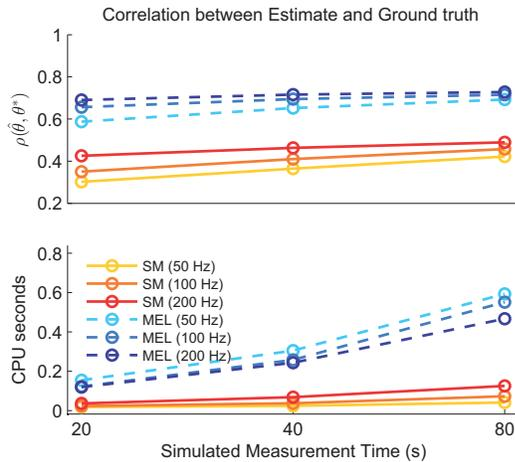
**Fig. 3.** Comparison between SM and maximum expected likelihood (MEL) estimation for a generalised quadratic model using Gaussian inputs. MEL offers clear advantages when expected likelihoods are computable with only modest computation burden.
