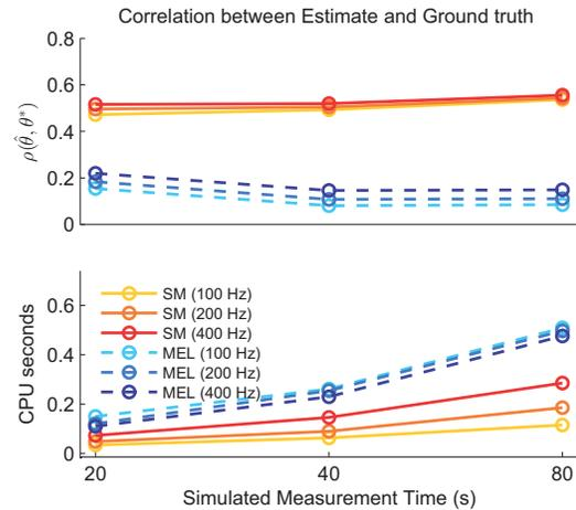
**Fig. 4.** Comparison between SM and MEL estimation for a generalised quadratic model using a speech signal input. Incorrectly computing expectations based on second order input statistics defeats the MEL approach as expected. SM remains robust (and, indeed, performs slightly better than with Gaussian noise).
