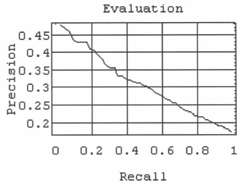
Figure 19: Average recall-precision curve for the Dice Coefficient using the corpus from Yahoo
