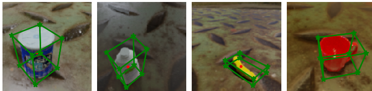
(c) Examples images from the YCB-Objects in-distribution test set shown with keypoint annotations. Each image is annotated with nine keypoints corresponding to the corners of the 3D bounding box and the object center. Models in the testbed predict these keypoints, and the object's 6D pose is recovered from keypoints using the PnP algorithm (Lepetit et al., 2009).
