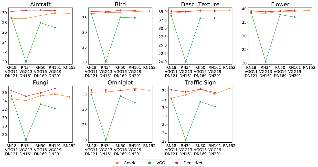
Figure 9. Scaling model size results. All models are trained on ImageNet and evaluated on the dataset marked top of each plot. X-axis lists each architecture variant with RN meaning ResNet and DN meaning DenseNet. Y-axis is the 5-way 5-shot accuracy. For 5-way 1-shot results, see Figure 8.
