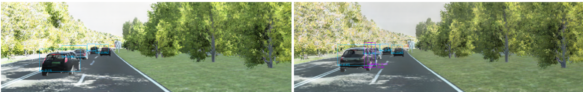
Figure 4. Semantic space adversarial examples. Benign re-rendered VKITTI image (top), adversarial examples generated by iterative sFGSM over a combination of semantic features (bottom). Cyan boxes indicate car detected, yellow indicates cyclist, and purple indicates pedestrian. The adversarial example introduces small changes in car positions and orientations, and noticeable changes in their color. This causes the network to detect pedestrians where there are none.
